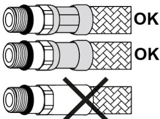
Before assembling the hose to the product ensure the hose ferrule has been crimped (as highlighted) on both ends of the hose after the braided hose sleeve.
