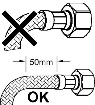
Both ends of the hose must have a minimum 50mm straight section before any bend.
