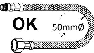
Observe the minimum bend radius of 50mm.
