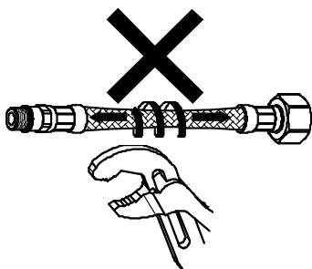
Never twist or stretch the flexible hose during installation.
