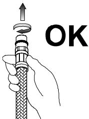
Always screw the flexi hoses into the product only by hand, until feeling mechanical rest, a spanner **must not** be used on the product end of the connecting hose.
