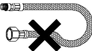
Hoses must not be double bent in multiple directions kinked or looped.
