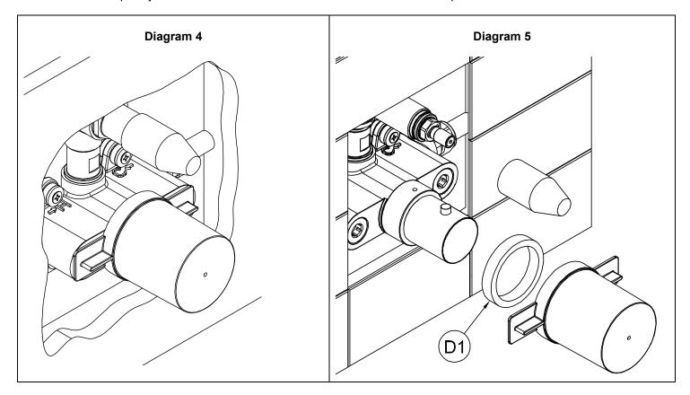
6. Make good the finished wall surface using tiles or similar, ensuring plastic valve caps (**C** & **D**) are in place as shown in **Diagram 4** to protect decorative parts. The tiles must overlap the finished shroud plate (**N**) by at least 15mm on each side of the plate. Do not tile over the inlet mesh filter ports (**A2**) and allow access to grub screw (Y).
