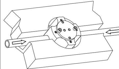
Turn the water feed on and check that there are no leakages before proceeding with the installation.
