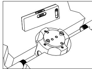
Check with a level that the built-in body is positioned flat and check that the depth of the built-in body is within its required parameters.
