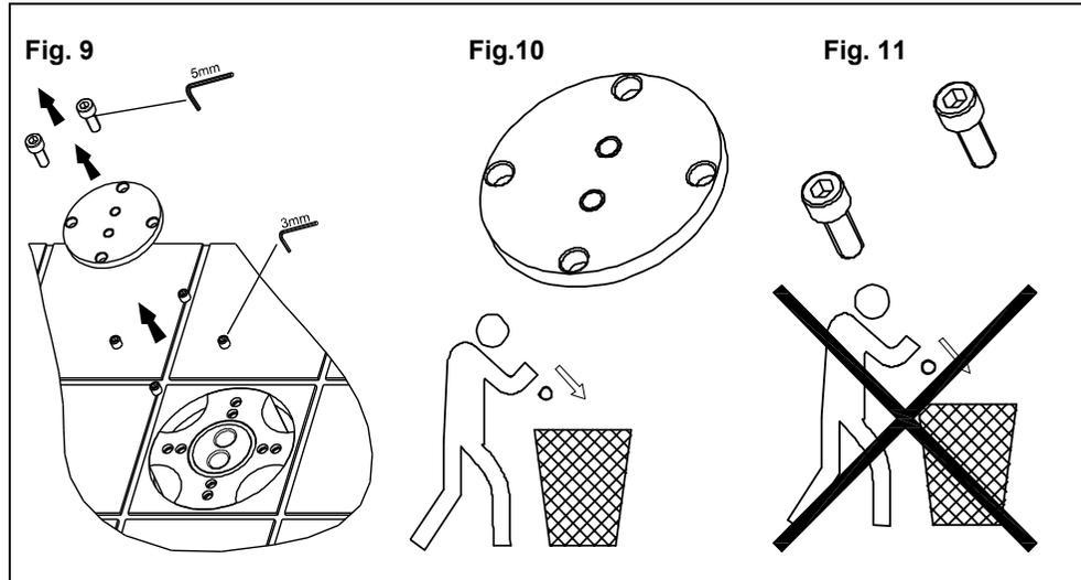
Remove the test plug by unscrewing the fixing bolts using a 5mm allen key.
