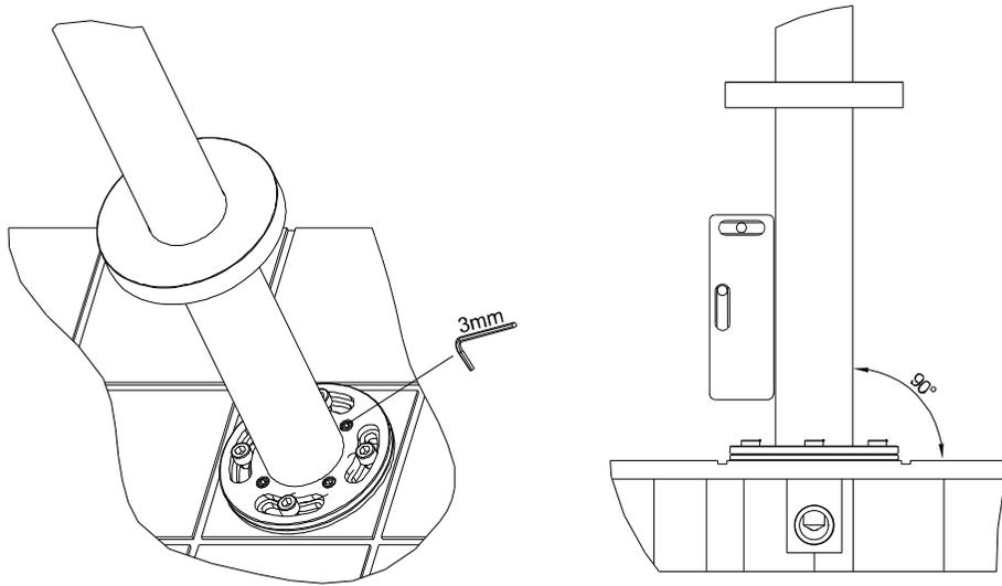
To ensure the bath filler is vertical the 4 x grub screws can be adjusted as shown above.
