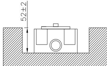
Create the seat for the body and for the supply pipes complying with the indicated sizes.
