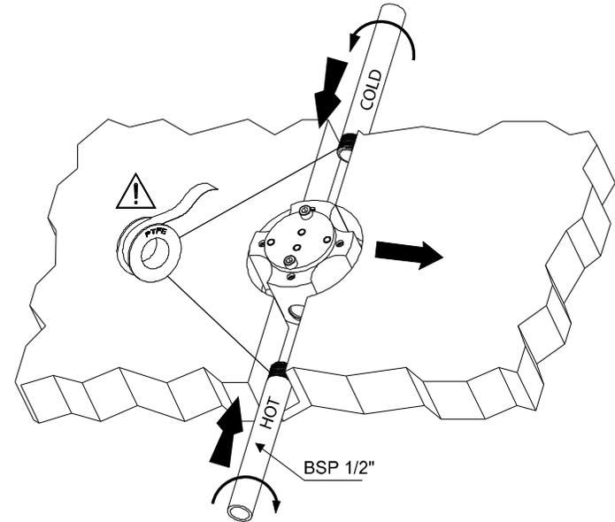
Connect the pipes to the body as indicated using Teflon or hemp to guarantee threads tightness. Isolation valves need to be placed in an accessible position for future maintenance (not below flow level).
