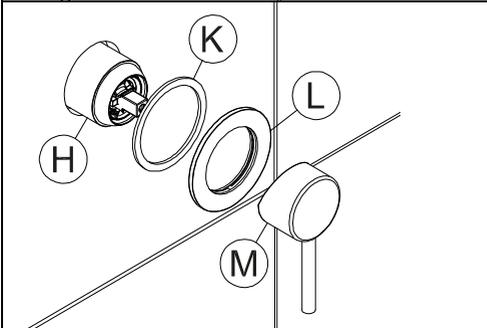
7. Insert foam seal (K) inside the back of back plate (L).
