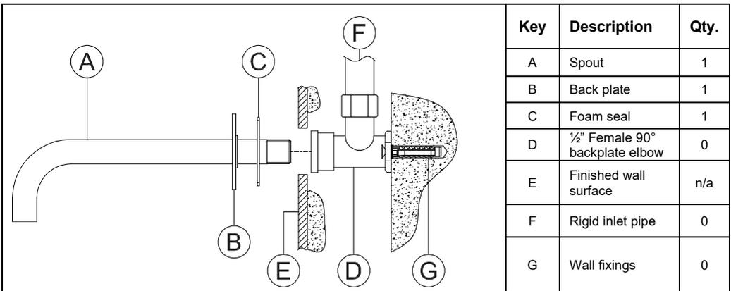
1. Open the wall / ceiling out to the required width and depth for supply pipe (F) and elbow (D).
