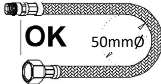
Observe the minimum bend radius of 50mm.
