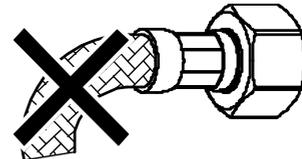
Both ends of the hose must have a minimum 50mm straight section before any bend.
