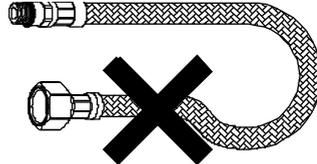
Hoses must not be double bent in multiple directions kinked or looped.
