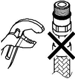
Always screw the flexi hoses into the product only by hand, until feeling mechanical rest, a spanner **must not** be used on the product end of the connecting hose.
