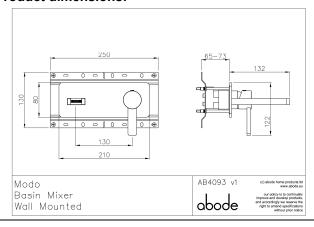
• Product mounted where: Wall • Recommended hole size: 190x60 mm
