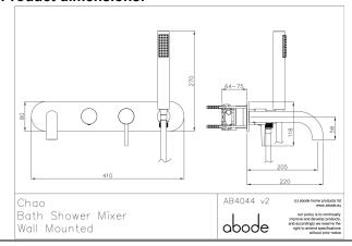
• Product mounted where: Wall • Recommended hole size: 390x60 mm
