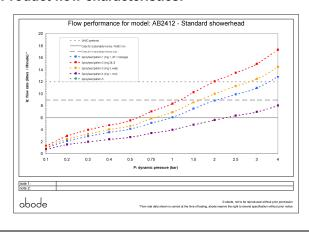
• Min / Max water pressure: 0.6 / 5 bar • Part G mixed flow rate at 3 bar (I/m): 14.95
