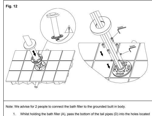
Whilst holding the bath filler (A), pass the bottom of the fail pipes (D) into the holes located in the built in body as shown.
