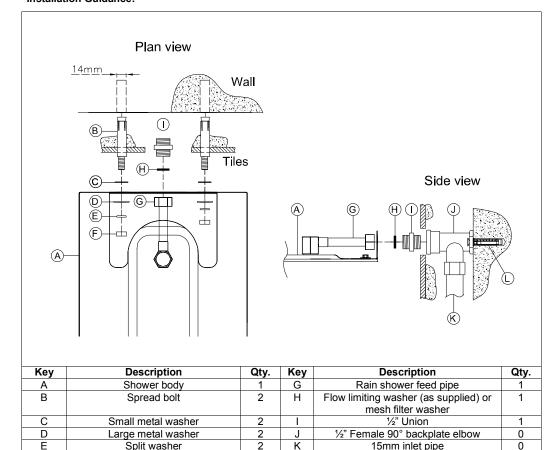
Note: A red 12 litre flow limiter is fitted between parts (G & H). This can be removed to improve the flow rate of the shower at lower pressures.
