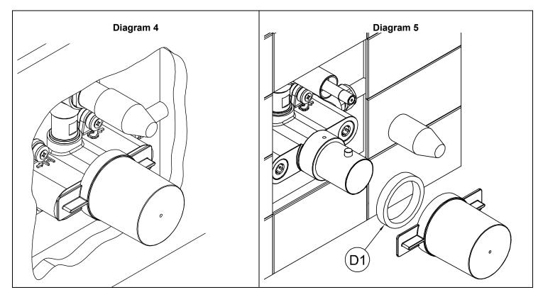
Make good the finished wall surface using tiles or similar, ensuring plastic valve caps (C & D) are in place as shown in **Diagram 4** to protect decorative parts. The tiles must overlap the finished shroud plate (N) by at least 15mm on each side of the plate. Do not tile over the inlet mesh filter ports (A2) and allow access to grub screw (Y).
